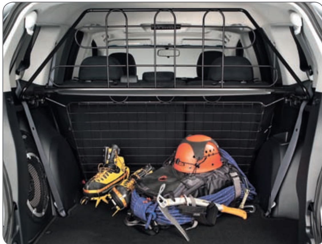
Separation rack ▶ Black-coated steel, roof to floor coverage. MZ314342
