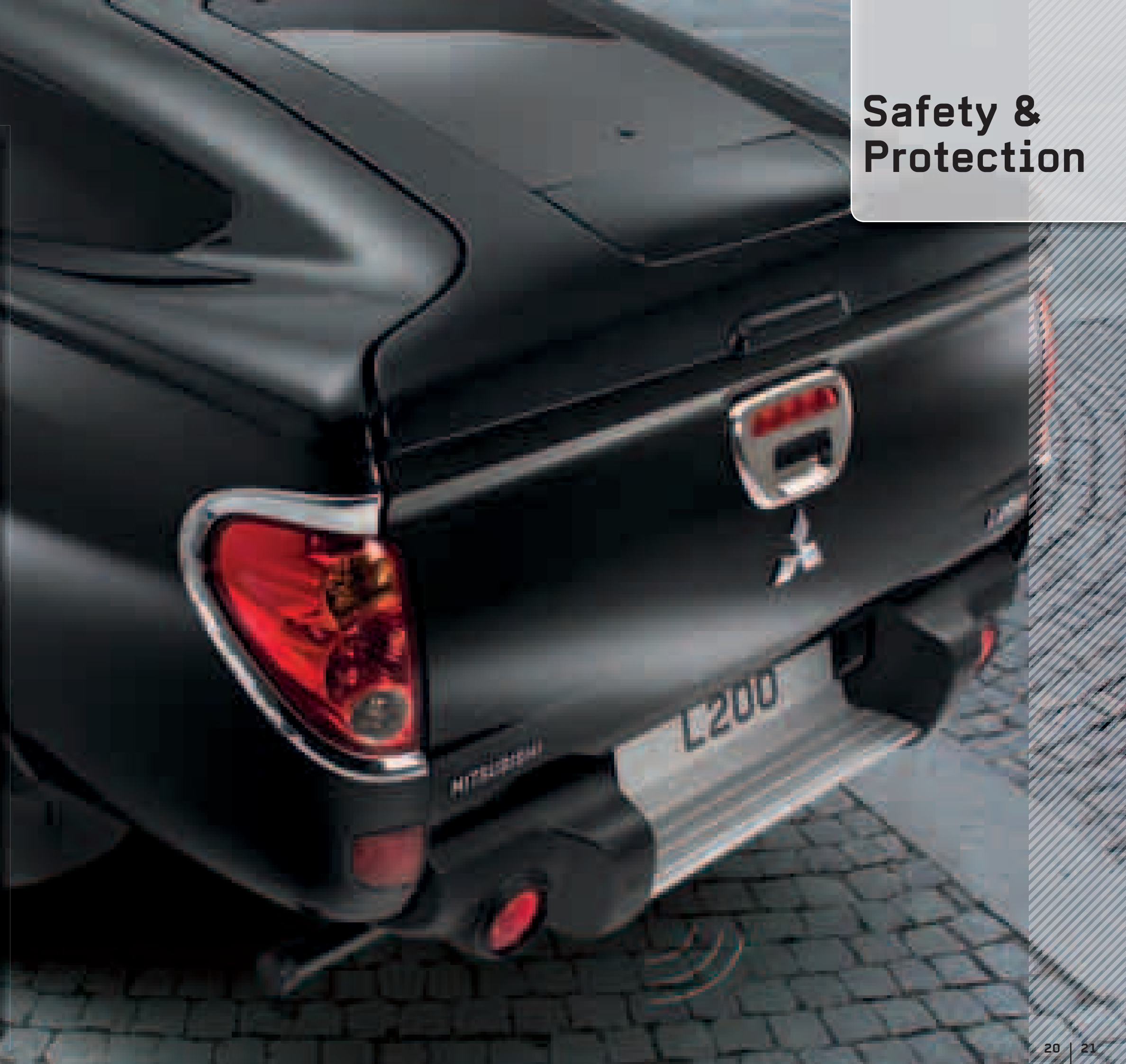
Rear parking assistance ▶ For vehicles with rear step bumper. 2 sensor-system, with audible distance indication.
